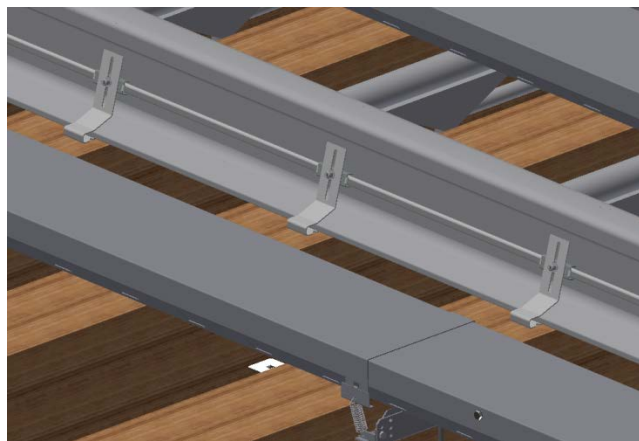
9226-1010 brackets installed along a rail
